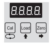
To begin the zero calibration, press the an and buttons together.
