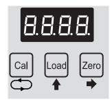
To begin the load calibration, press the 💷 and Load buttons together.
