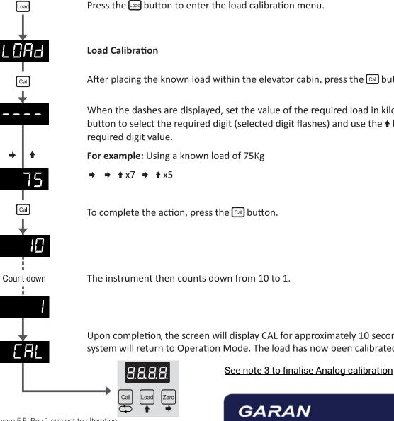
After placing the known load within the elevator cabin, press the 🖾 button to proceed.
