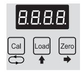
To begin the zero calibration, press the a and a buttons together.
