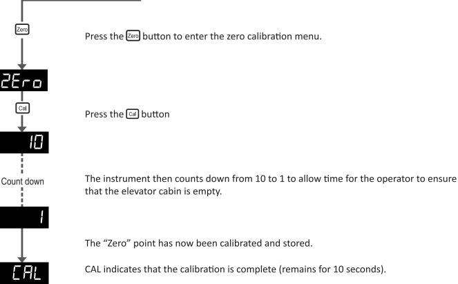
Press Im within 10 seconds to proceed to the Load Calibration.
